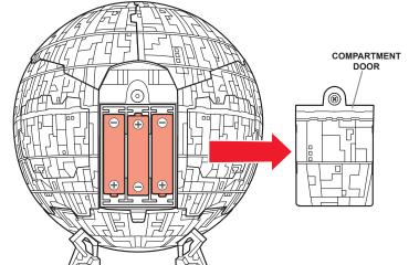
Using a Phillips/cross head screwdriver (not included), loosen screw in battery compartment door (screw remains attached to door). Remove door. Remove exhausted batteries and insert 3 x 1.5V "AAA" or R03 size batteries (not included). Alkaline batteries recommended. Replace door and tighten screw.
